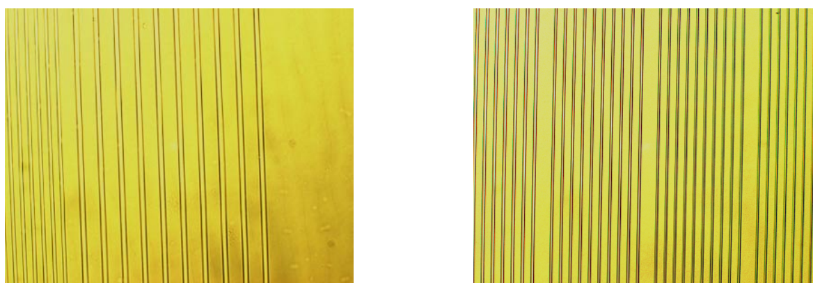
Figure 7.7 Two microscope photographs that show a part of the ridge waveguides with different thickness.
